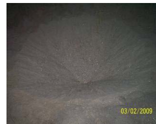
Pits getting filled up by dugout sand due to impact of high velocity wind at Kataiya (Basantpur, Supaul)
